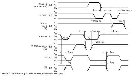
Note B: Prior to test, HIGH level data is loaded into the P7 input.
